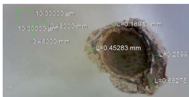
Fig. 4. Thickness of the layer of Scots pine seed ( Pinus silvestris L.) at the first stage of pelletizing (time - 7 minutes)
