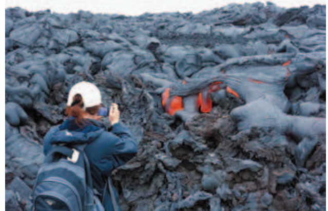
Fig. 4. Temperature at a point in red hot lava measured with an emission pyrometer was 650-700 °C.
